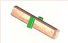
7 Cant turner DV 56-1 90° cant turning
