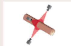
2 3D-scanner Round log scanning
