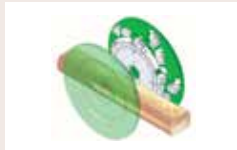
8 Chipper canter VM 45 Resawing of two-sided cants, production of four-sided cants and chips
