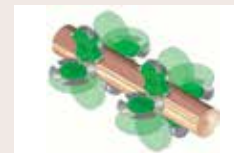
4 2x Profiler unit VPM 450/N Profiling of two sideboards diagonal to the cant support
