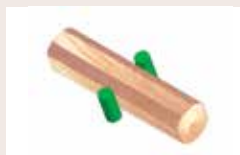
8 Cant turner DV 70 90° cant turning
