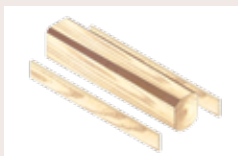
9 Separating conveyor SEB Sideboard separation
