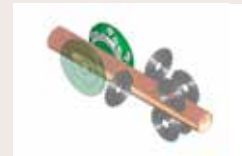
2 Chipper canter VM 50 Opening of two log faces, production of two-sided cants and chips
