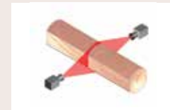
5 Two-sided cant scanner Sideboard re-optimization
