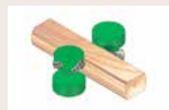
14 Profiler unit VPF 340 Profiling of two sideboards
