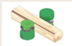
11 Profiler unit VPM 450 Profiling of two sideboards
