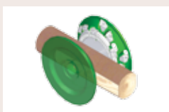
2 Chipper canter VM 45 Opening of two log faces, production of two-sided cants and chips
