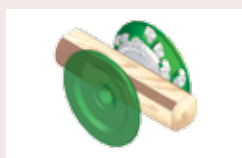
4 Chipper canter VM 45 Opening of two faces, pro- duction of four-sided cants and chips
