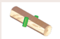
3 Cant turner DV 70 90° turning of two-sided cants
