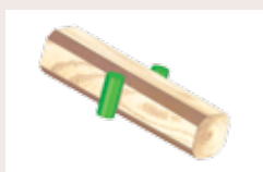
5 Cant turner DV 70 90° turning of four-sided cants
