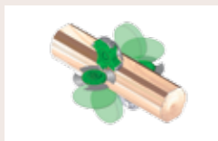
12 Profiler unit VPM 450 Profiling of two sideboards
