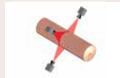
1 3D-scanner Round log scanning
