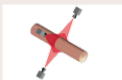
1 3D-scanner Round log scanning
