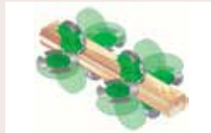
9 2x Profiler unit VPM 450/5 Profiling of two sideboards
