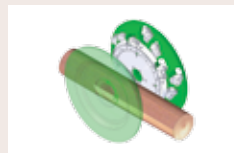
3 Chipper canter VM 45 Opening of two log faces, production of two-sided cants and chips
