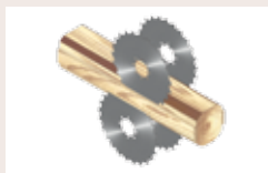
8 Saw unit CSMK 285-A1/B1 Resawing of two-sided cants, production of four-sided cants and sideboards
