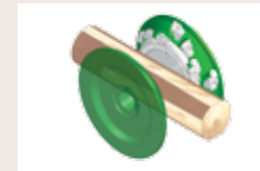
4 Chipper canter VM45 Opening of two faces, production of four-sided cants and chips
