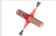
1 3D-scanner Round log scanning
