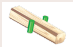
10 Sideboard separation 90° turning of four-sided cants
