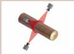
1 3D-scanner Round log scanning
