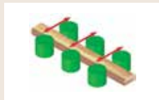
8 Infeed- and centering system EVP45 SZ-Z3 Automatic cant centering or diagonal alignment
