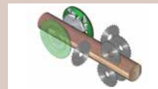
2 Chipper canter VM50 Processing of round logs, production of two-sided cants and chips
