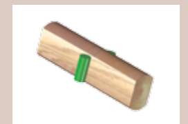
6 Cant turner DV90 Turning of two-sided cants by 90°
