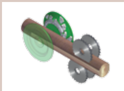
3 Chipper canter VM45 Processing of round logs, production of two-sided cants and chips
