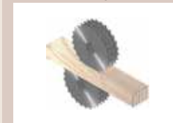
5 Circular resaw CSMK225-A1 Resawing of four-sided cants
