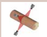
1 3D-scanner Round log scanning
